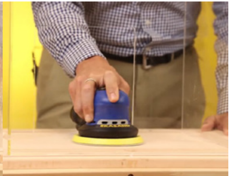
Sanding with dust extraction
